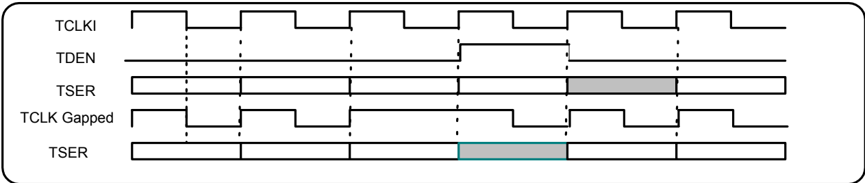
Figure 10-1 TX Serial Interface Functional Timing
