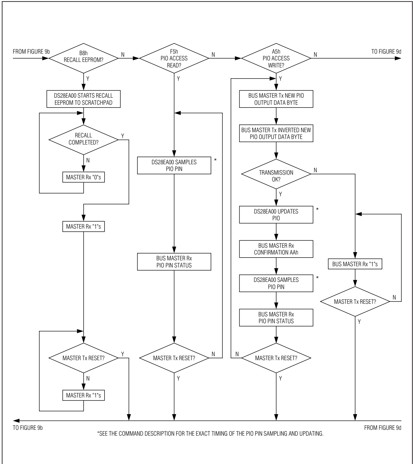
Figure 9c. Control Function Flowchart
